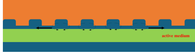
Fig 6. Waves travelling in a DFB laser
