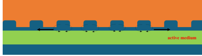
Fig 6. Waves travelling in a DFB laser
